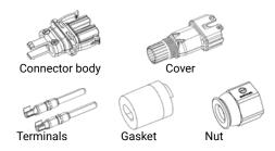
★ WARNING: Risk of equipment failure. Do not mix male and female connector parts when assembling connectors.
